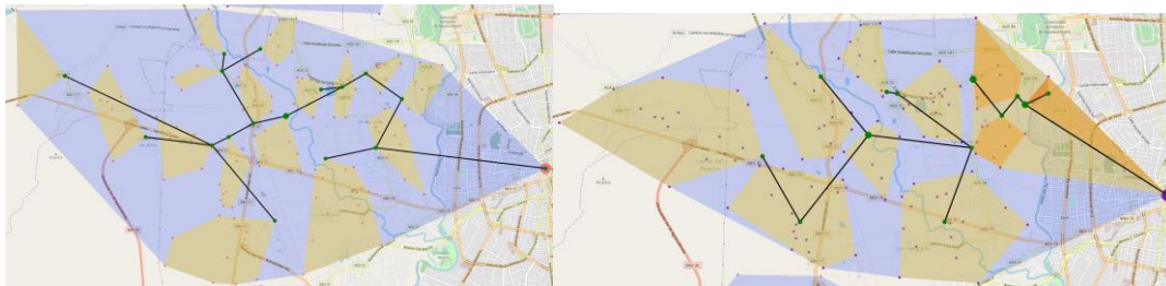
Figure 5. Left network topology without distance to road, Right network topology weighted with distance to road
